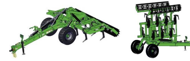
The ThunderRipper® by K-Line Ag is a heavy-duty yet compact ripper designed to break up compacted soils and improve root penetration. With tines capable of reaching a depth of approximately 450-500mm, the ThunderRipper® promotes better plant development by facilitating the entry of nutrients and moisture, as well as enhancing the accumulation of organic materials in the soil.
